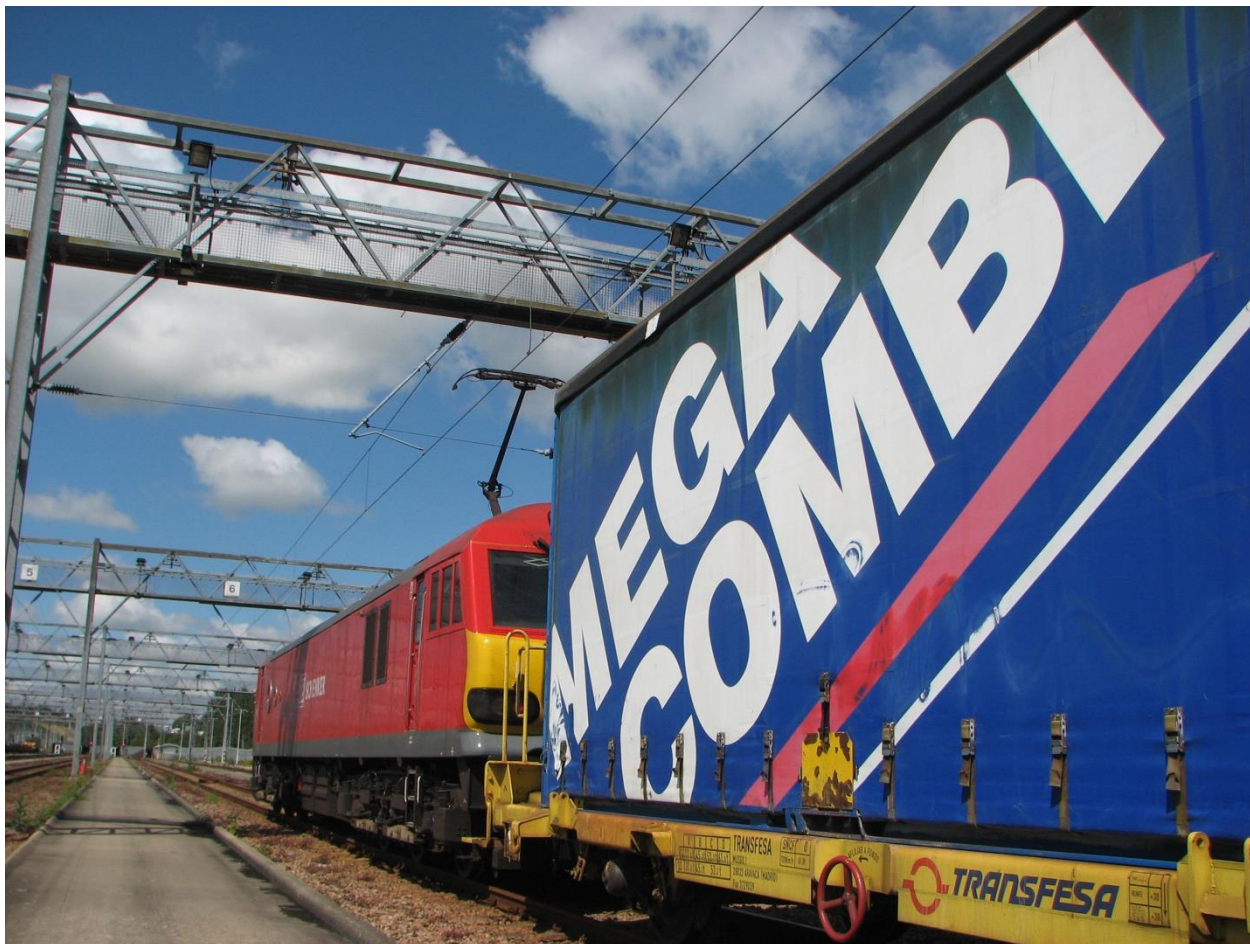
Figure 4.3 – Softsided Swap Body with Bottom Lift points
